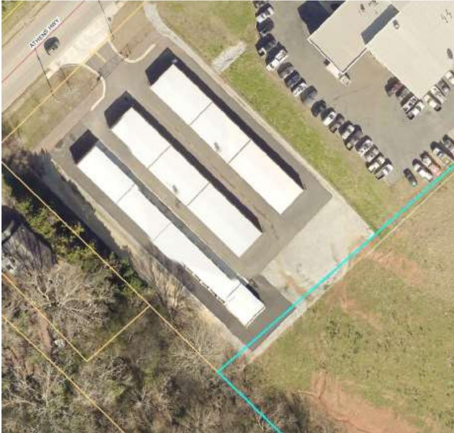
A closer aerial photograph showing the existing mini storage buildings and the paved driving/parking areas around the units (darker grey). There is a gravelled area in the back of the buildings (lighter grey).
